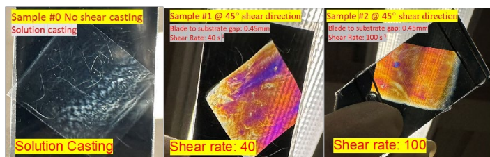
Fig.1 Shear casting P(VDF-HFP)-CNC (30 wt.%) composite under cross polarized
